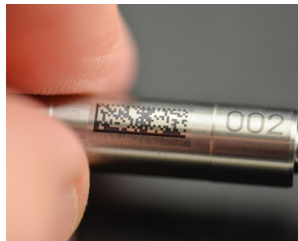
Annealing on stainless steel
