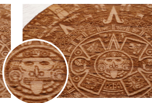
4.0" engraving A rough engraving that looks blurred
