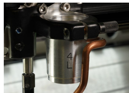
Lens 4.0" Thick cutting and fast engraving
