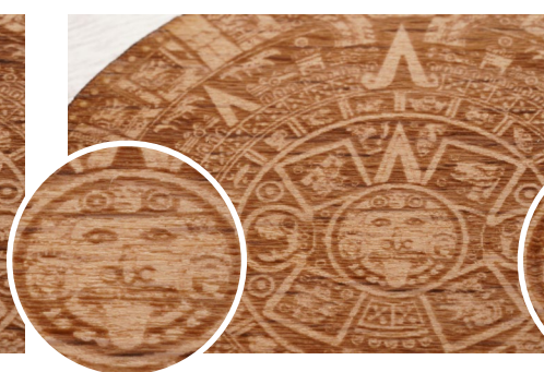
2.0" engraving A fine result but some small details are missing
